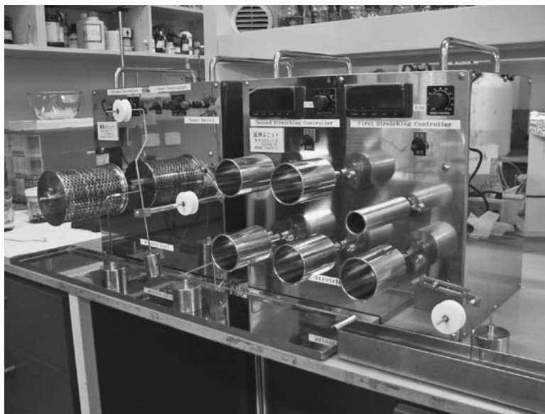
FIGURE 7.9 The customized wet-spinning apparatus at the Intelligent Polymer Research Institute, University of Wollongong.
